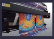
Inline X & Y-directional cutting is possible. The system reads the dedicated registration marks and automatically cuts the sheets. dramatically reducing labor and optimizing all post-processing.
